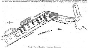
separated by sand dunes from the sea, as at Calais, Dunkirk (fig. 6) and Ostend (see HARBOUR). In sheltered places on the sea-coast, docks have sometimes been constructed on lowlving land bordering the shore, with direct access to the sea, as at Barrow and Hartlepool; whilst at Mediterranean ports open basins have been formed in the sea, by establishing quays along the foreshore, from which wide, solid jetties, lined with quay walls, are carried into the sea at intervals at right angles to
